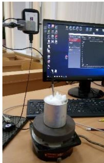
$$\lambda = C_B \frac{m_B(t_B - t_{кон}) - m_L(t_{кон} - t_L)}{m_L}$$
